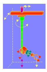
The virtual reality model represents a nuclear hot chamber manipulator. It is manipulated by a simple Simulink model containing the Space Mouse Input block. This model uses all six degrees of freedom of the space mouse for manipulating the mechanical arm, and uses mouse button 1 to close the grip of the manipulator jaws.
